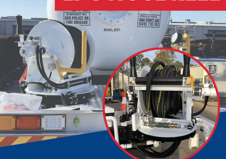
Model E8037 **Turntable Style** Hose The AGI Reel, manufactured by Air & Gas Industries, is configured with a turntable mount allowing it to make deliveries on either side and to the rear of the vehicle.
