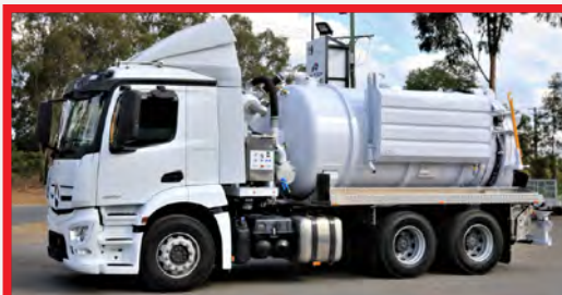
6X4 HYDRO-EXCAVATION TRUCK 11,000 LITRE VESSEL
