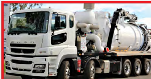
8X4 OR 10X4 HYDRO-EXCAVATION JETTER TRUCK 11,000-13,500 LITRE VESSEL
