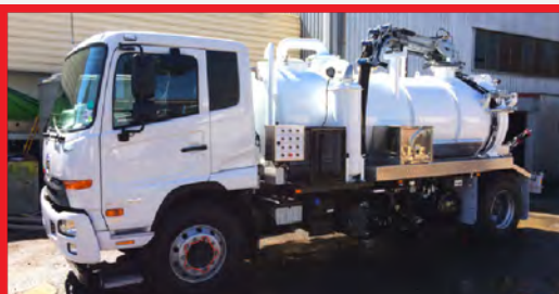
4X2 HYDRO-EXCAVATION TRUCK 6,000 LITRE VESSEL
